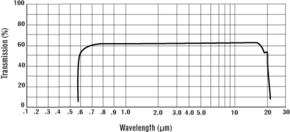
Figure D4.1.3: transmission of ZincSelenide in through the IR range
