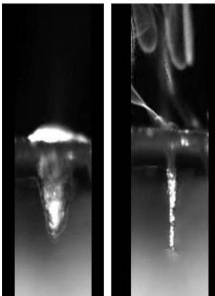
*Figure D4.1.7: Example of imaging tissue ablation at 10.000 frames/sec: (left) Ablation of transparent tissue model showing the expansion of the ablation crater during vaporisation of the tissue. (right) After the laser pulse, the crater collapses and steam/aerosols are ejected. The scale of the images is 2 x 8 mm.*
