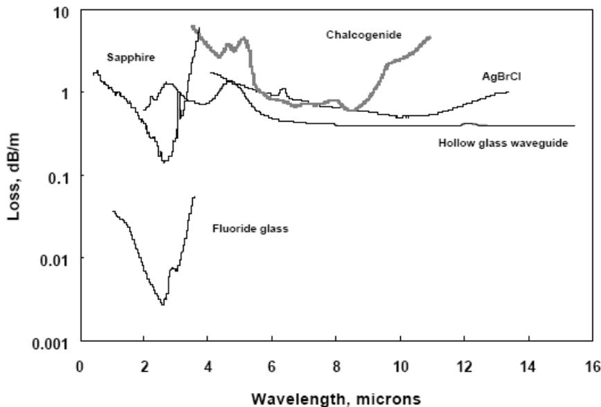
Figure D4.1.5: Typical transmission losses of the materials used for IR fibers.
