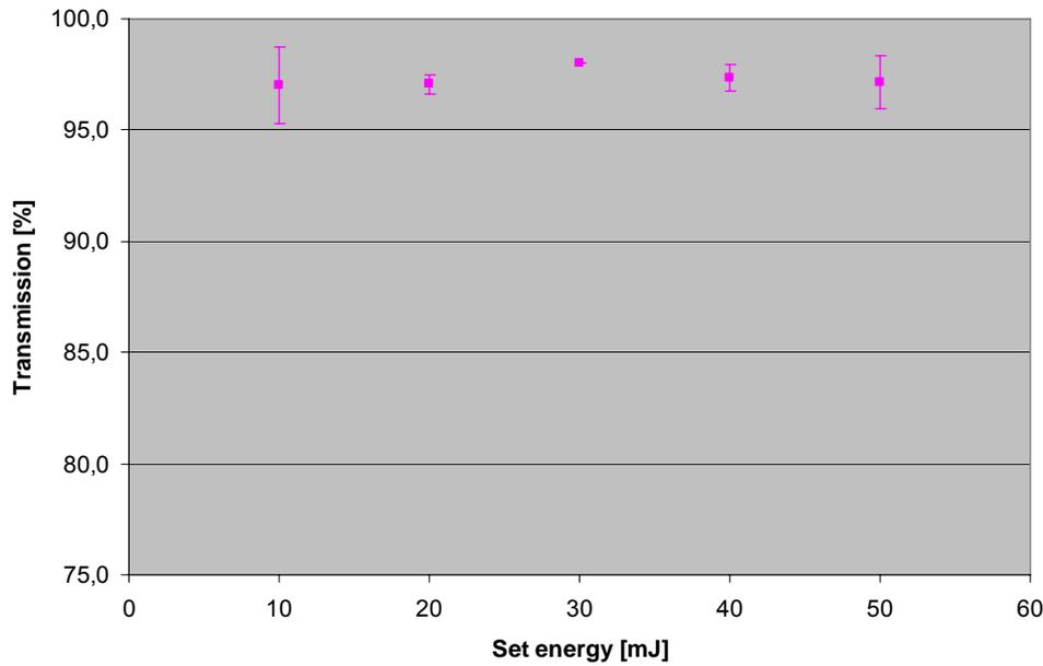
Figure D4.1.6: transmission through a 1000 μm bore diameter HWG with a length of 550 mm
