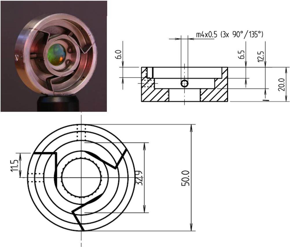
Figure D4.1.2: photo and drawings of back side of entrance with lens holder and x-y positioning system
