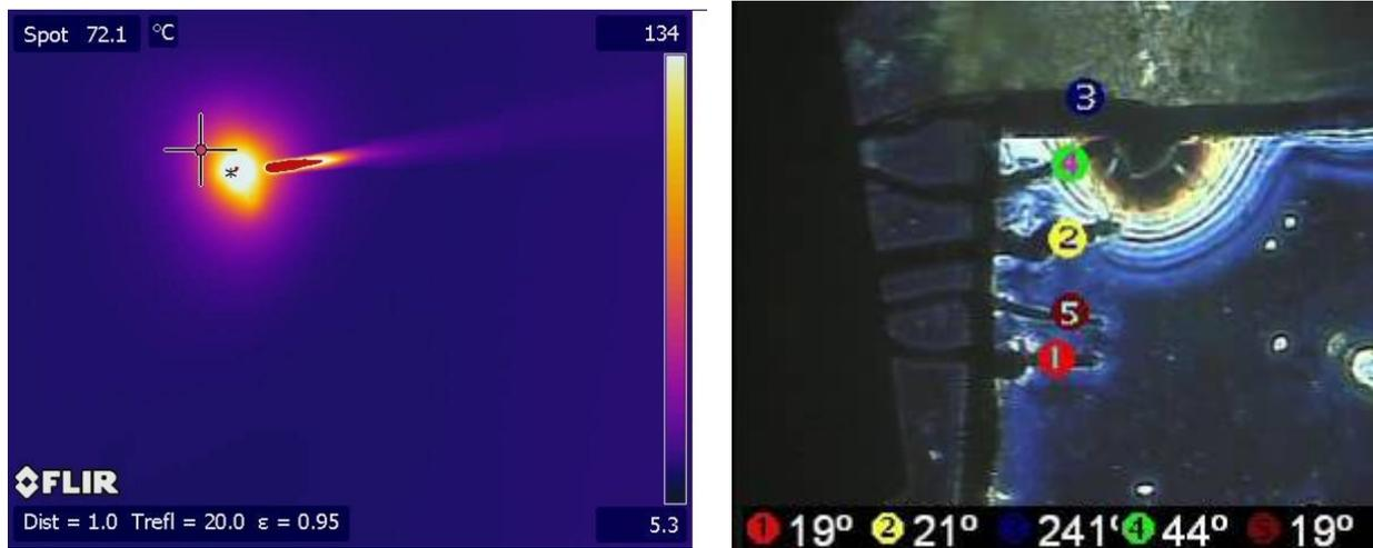
Figure D4.1.8: Examples of thermal images during laser exposure of tissue. Left: Image obtained with a thermal camera showing the hot spot on tissue irradiated by a laser light from a fiber. Right: Image obtained with a Color Schlieren Technique showing temperature gradients around the ablation crater from the side in a transparent tissue model. The absolute temperatures are measured with thermocouples and superposed on the bottom of the image.
