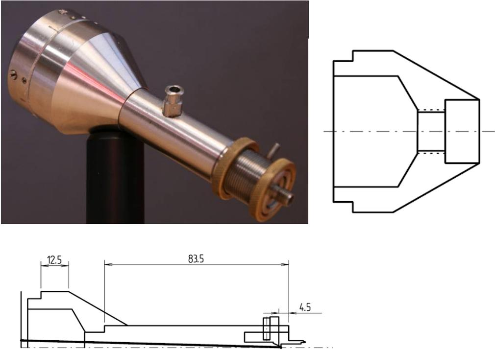
Figure D4.1.4: photo and drawings of the SMA fiber coupling side
