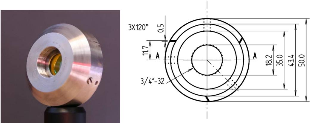
Figure D4.1.1: photo and drawing of front side of entrance of the coupler
