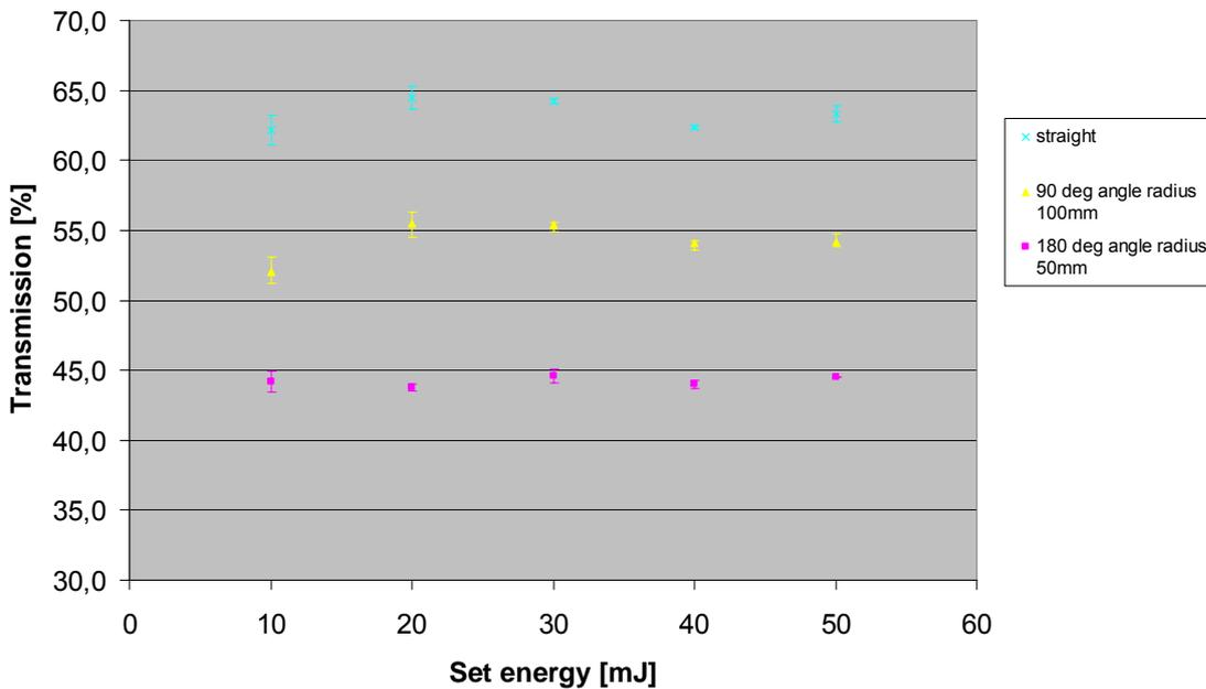
Figure D4.1.6: transmission through a 320 μm bore diameter HWG with a length of 800 mm for the conditions: straight, 90 degree angle bend and 180 degree angle bend.
