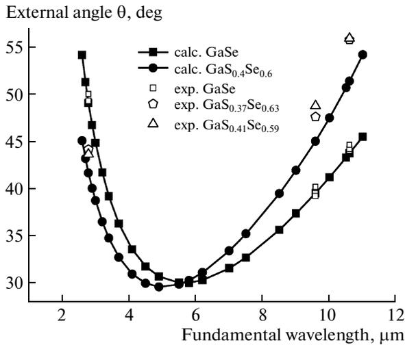
Fig. 5. SHG phase-matching in GaSe and  $\text{GaS}_x\text{Se}_{1-x}$ : calculation and experimental data from [8] (open symbols).
