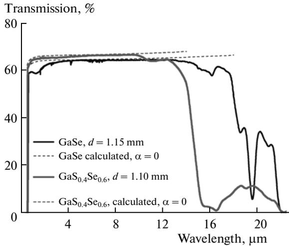
**Fig. 3.** Full measured transmission of GaSe and GaS<sub>0.4</sub>Se<sub>0.6</sub> for *o*-polarization (thick lines), and theoretical calculation taking into account multiple reflections (thin lines).
