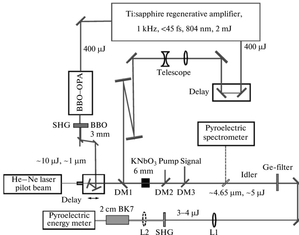
Fig. 6. Experimental setup for relative measurement of the SHG efficiency: DM, dichroic mirrors, L, lenses.
