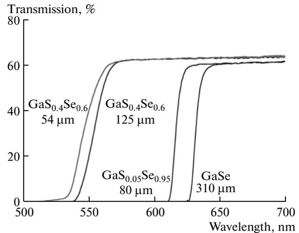
**Fig. 2.** Transmission of some  $\text{GaS}_x\text{Se}_{1-x}$  mixed crystals close to the band-gap ( $o$ -polarization).
