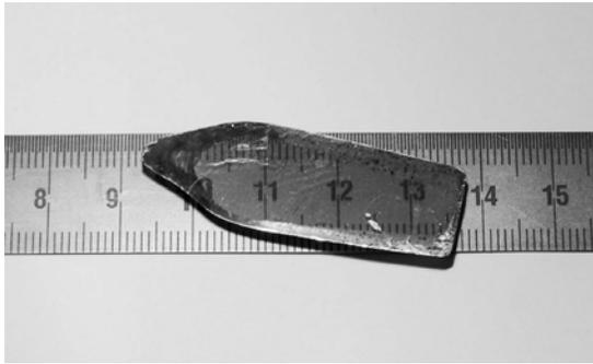
**Fig. 1.** Cleaved plate from an as grown crystal of  $\text{GaS}_{0.4}\text{Se}_{0.6}$  with a thickness of 3.5 mm.
