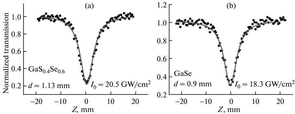
**Fig. 7.** Open-aperture  $z$ -scan signals of  $\text{GaS}_{0.4}\text{Se}_{0.6}$  (a) and  $\text{GaSe}$  (b) with fit curves.  $I_0$  denotes the peak on-axis intensity incident on the samples.
