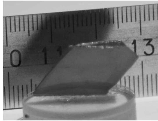
**Fig. 4.** Prism of GaS<sub>0.4</sub>Se<sub>0.6</sub> used for measurement of the two refractive indices.
